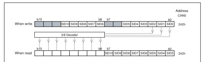
Figure 18.19 Write/read of COAFS Register in Word Access
